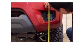
11. On your vehicle, measure the distance between the ground and the center of your SS3 pod. This is your mounting height.
