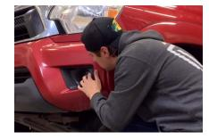
10. Loosen the 5/32" allen bolts on each side of your SS3 pod, just enough to allow you to adjust the pod.
